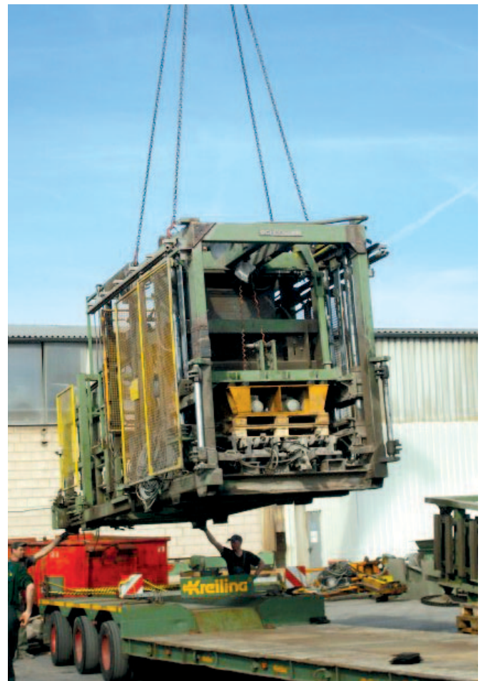
Loading of dismantled Schlosser SV 30 blockmaking machine on a deep bed loader
